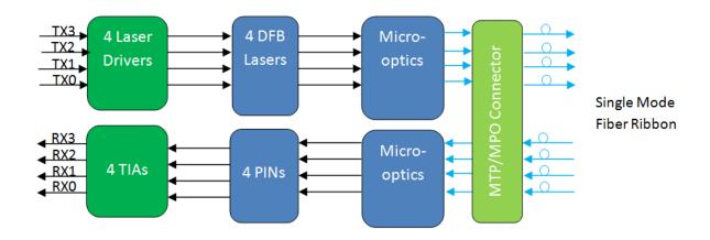
Figure 1. Transceiver Block Diagram
