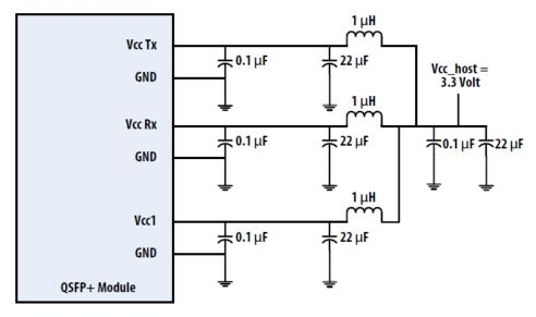
Figure 3. Recommended Power Supply Filter
