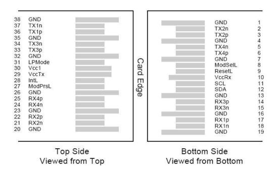
Figure 2. QSFP28 Transceiver Electrical Connector Layout
